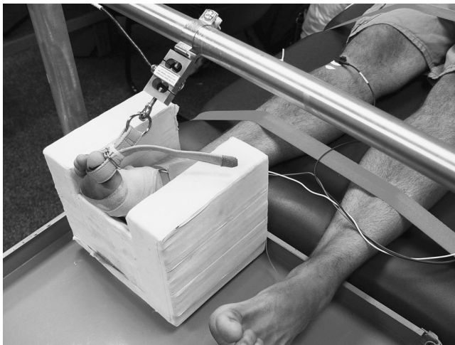
FIGURE 1—Great toe harness and strain gauge attachment.
